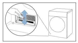
**Note:** Always clean the fins on the heat exchanger from top to bottom, taking care not to bend or damage them.
