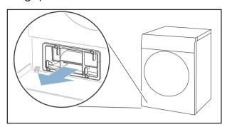
**5.** Carefully remove the filter mat from the heat exchanger cover.
