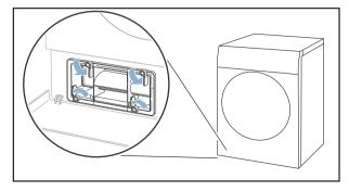
**4.** Pull the heat exchanger cover out by its grip.
