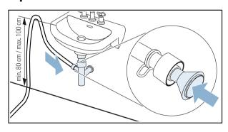
The connection point must be secured using a hose clamp (12-22 mm clamping range, available from specialist retailers). When connecting to a siphon, make sure that the drain hose is routed at a height of at least 80 cm, but no more than 100 cm.
