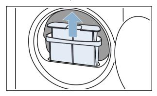
3. Remove the fluff from the fluff filter recess. Ensure that no fluff falls into the open shaft.
