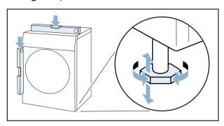
3. If necessary, turn the appliance feet to make sure it is level.
