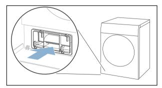
**Note:** You can only slide the heat exchanger cover in if the insert is in the appliance.
